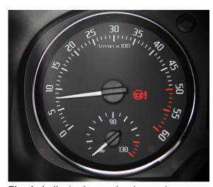
Fig. 1: Indicator lamp, steering system
