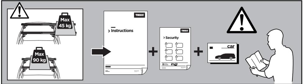
**GB** Maximum load Thule SlideBar = 45/90 kg, or less if stated differently in roof rack- or car instruction manual.
