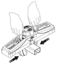
Push together until both hooks meet roofrack.
