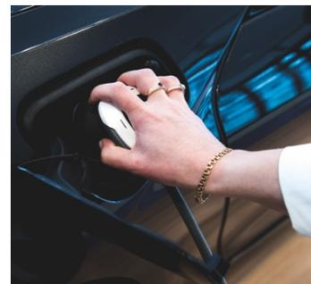
Open the latch by placing your palm on the connector
